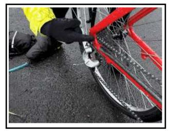
Shift rear derailleur to smallest cog. Move QR to open position or loosen axle nuts
