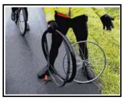
4. Remove the tube from inside the tire.
