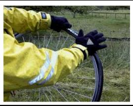
4. Starting from the valve stem, with both hands, roll tire onto rim. Work evenly in both directions from the valve stem. When Tire becomes tight, hold tire and wheel in upright position. Twist and push tire in a downward motion. Rotate wheel and continue rolling tire onto rim. Never use tire levers or screwdriver to mount the tire because this will pinch the tube.
