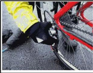
Pull the body of the derailleur towards the back of the bike so that the axle can clear the derailleur - remove wheel
