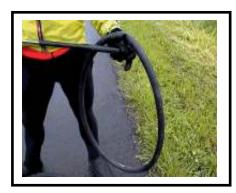
4. Inflate tube to make sure patch is secure and that air does not escape.
