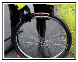
3. Place one side of the tire on the rim and the valve stem through the hole in the rim. Mount directional tires according to arrow on the sidewall.
