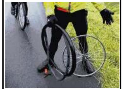
**4. Remove the tube from inside the tire.**
